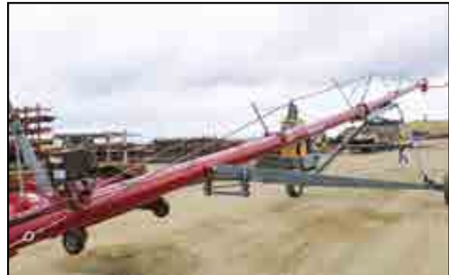
Fig 19 - Upward bow in auger tube
