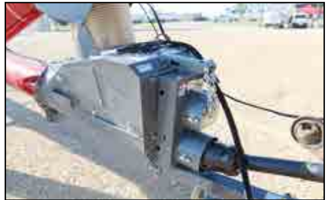
Fig 5 - 13" Auger boot with 540 PTO driveline
